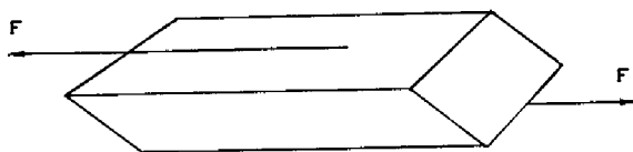
Fig. 7.2—Bar under shearing stress
