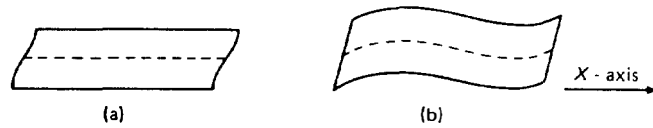
Fig. 9.5. Edge view of the strains in an AT-cut plate (a) vibrating in thickness shear and (b) vibrating in its first even flexure mode.
