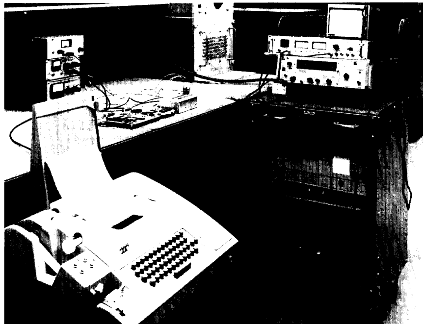
Figure 10-26. Test setup for microprocessor temperature compensation.
