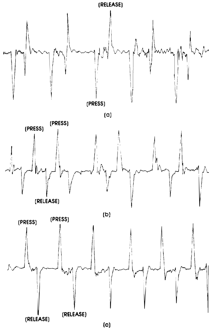
Figure 4.3 Strip chart recordings of press test measurement (Figure 4.2) for lithium niobate: (a) press y measure along y determines d_{22} ; (b) reversing the electrodes reverses the sign of the voltage; (c) press x measure along y determines d_{21} = -d_{22} .
