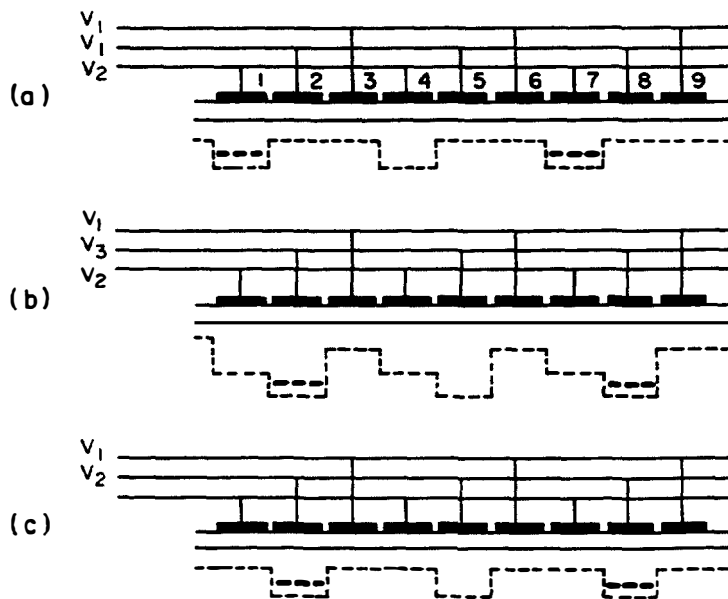
Figure 4.3.6 Three-phase CCD; illustration of its operation.
