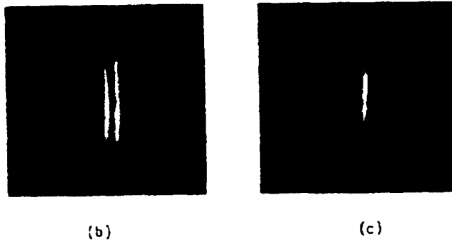
Figure 3.5.33 Pitch/catch imaging: (a) transmitter-receiver geometry and diagram of the three waves scattered from the crack; (b) pitch/catch image of a long 7-mm-deep slot; (c) pitch/catch image of the 10-mm-long fatigue crack. (After Kino et al. [49].)
