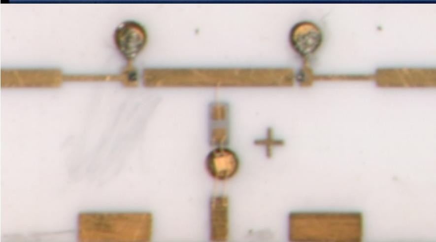
3-6GHz resonator (5mm) on alumina
