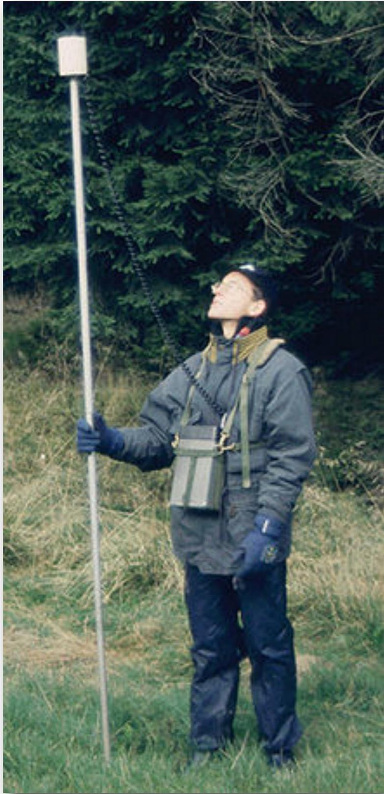
Measurement of weak magnetic field (like Earth's field, with  $\mu_0$  used for calibration)
