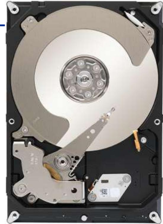
*“The actuator arm and suspension of the rotary actuator are collinear making the movement of the slider follow an arc and not a straight line.”*
