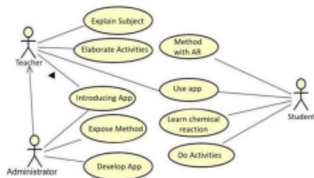
Fig. 2 - Use Case Diagram of the Proposed System.
