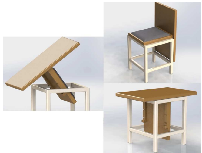
Fig. 2. Project 2: virtual prototyping using Solidworks of a multi-purpose furniture item. The designed item can be a chair or a table.
