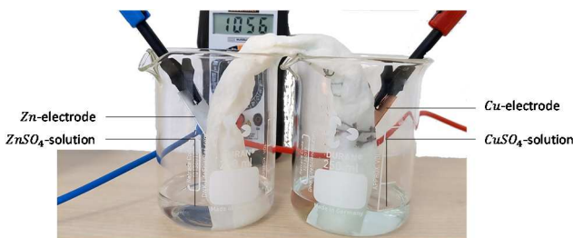
Fig. 7. Experimental accumulator set-up
