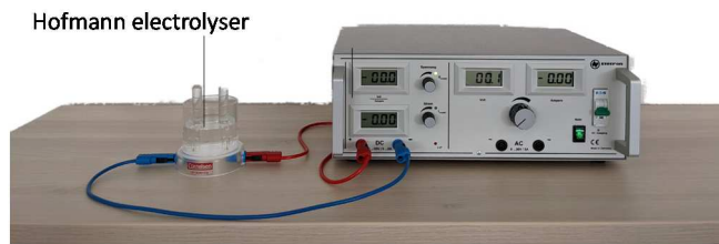
Fig. 3. Experimental electrolyser set-up
