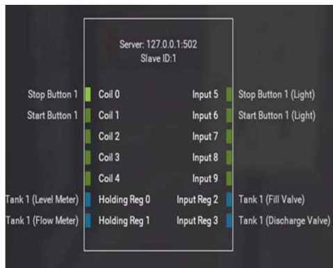
Figure 17. Factory IO virtual PLC showing input and output connections for sensors and actuators.
