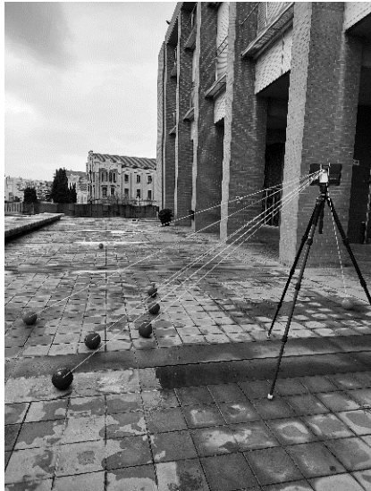
Fig. 3. LIDAR. scanning the scene with the TLS.
