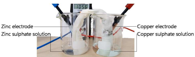
Fig. 5. Daniell-cell accumulator experiment [11]
