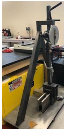
Figure 3. Impact Tester (Charpy)
