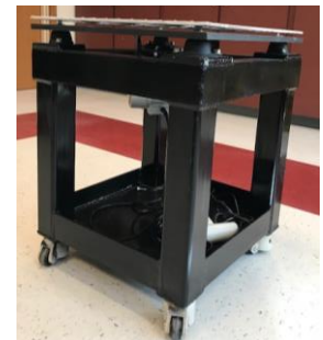
Figure 7. Concrete Vibration Compaction Machine
