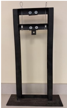
Figure 2. Creep Tester
