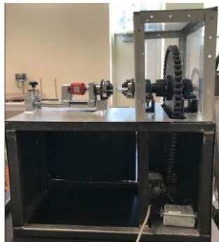
Figure 4. Torsion Testing Machine
