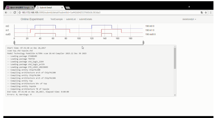
Fig. 5. The simulation waveforms of a submission
