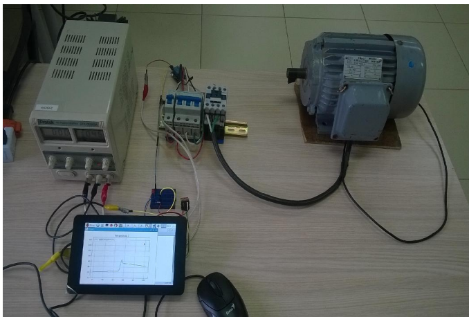
Fig. 5. Design 2. The students designed an emergency stop for the ACIM and they plotted the temperature sensed by the device TMP102 through Matplotlib in Python.
