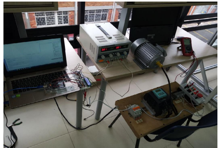
Fig. 6. Design 3. The students configured the parameters of the variable speed drive Sinamics G110. The speed was handled through a digital potentiometer in the Arduino Mega 2560.
