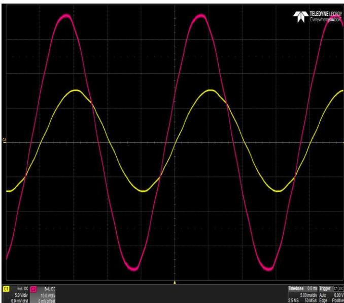
Fig. 5. Line voltage on the primary and secondary sides of Figure 4.
