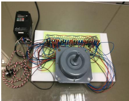
Fig. 7. Supply three-phase input voltage to the induction motor.
