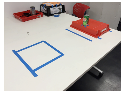
Fig. 2. The test setup. Robots start at the left of the test setup, retrieve the can from the platform on the right, and deposit the can in the box on the left. The lines to the left of the taped box and platform serve as guides to help students position their robot.
