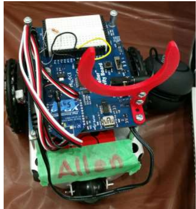
Figure 2. The 3D printed speaker support mounted on an Activitybot.
