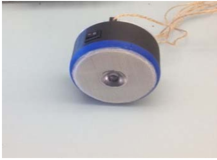
Fig. 9. Solar PV lantern for Team 2. (Project IV)
