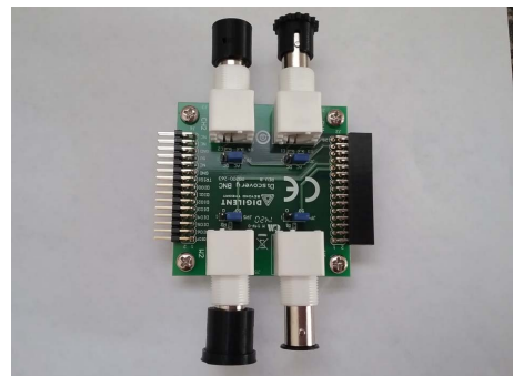
Fig. 2. Design caps exactly fit the BNC ports.
