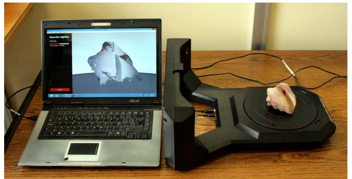
Fig. 4. Scanning process of a fossil using MakerBot Digitizer
