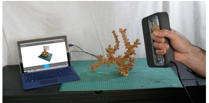
Fig. 3. Scanning process of a coral using Sense 3D scanner
