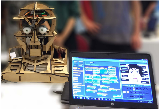
Fig. 1. Animatronic built and programmed by Scratch
