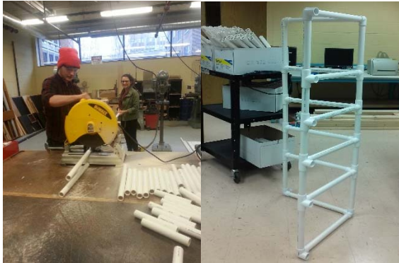
Fig. 6. Cutting station where students cut the PVC pipes to piece with different length and one segment of the planter
