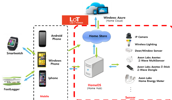
Figure 1. Interconnection of a LoT system
