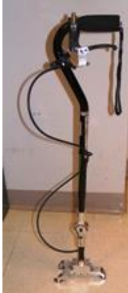
Fig. 3. Combination of a free standing cane and grabber.
