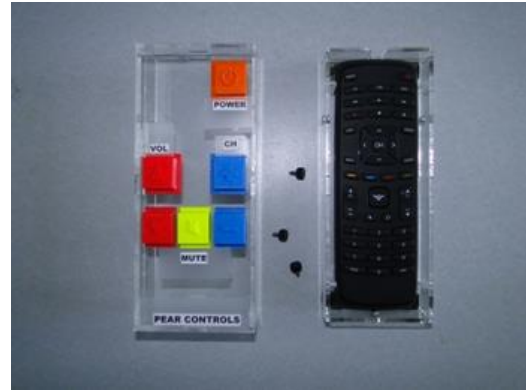
Fig. 1. A case for a TV remote that makes it usable for persons with cognitive and physical disabilities.
