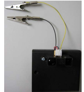
Fig. 3. Assembled IR-based sensor "Radar" system prototype.
