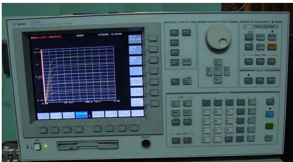
Figure 2. Experimental setup for semiconductor device characterization. BJT output characteristics is visible on the instrument's screen.
