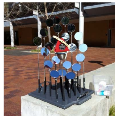
Fig. 3. Sterling engine powered by solar energy. The design challenge for the students is to determine the optimum position for the mirrors.
