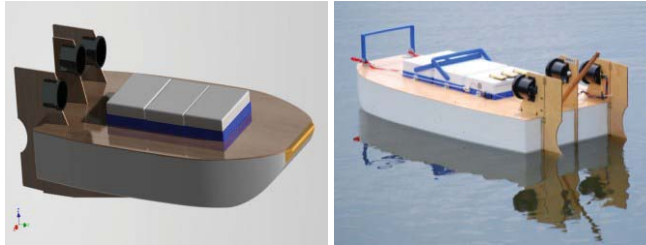
Figure 2a: CAD solid model Figure 2b: R/C ROVER X-2 forward operation, and deflect water in reverse mode. For the initial phase, a LABQUEST 2 interface [2] was utilized to collect geo-located water quality data such as salinity, pH, dissolved oxygen (DO) and temperature with Vernier sensors [3] on the boat (Figures 3a and 3b). Subsequently,
