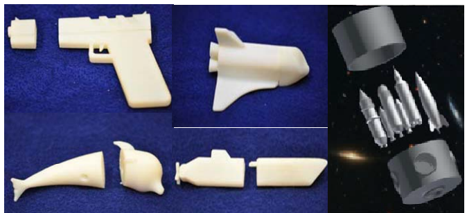
Figure. 2. Example flash drive cases printed on an Objet rapid prototyper (left and middle). Example set of flash drives and a case based on the space program (right). The case was designed to mimic a segment of the international space station.
