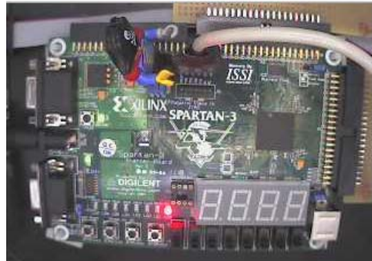
Fig. 22. FPGA board through the experiment's webcam
