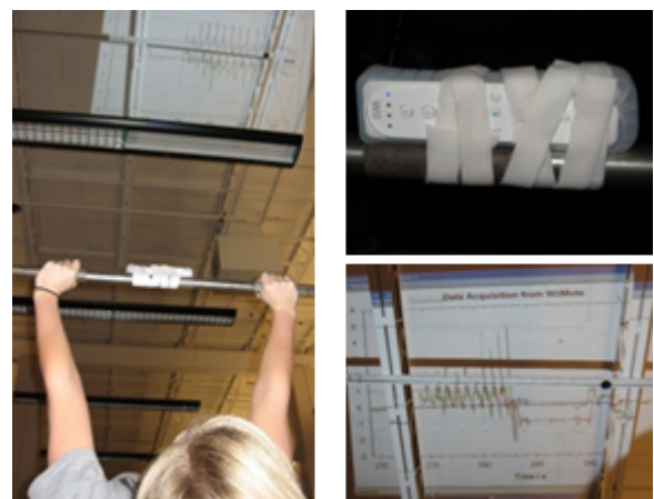
Fig. 9. A WiiMote mounted to a bench-press bar, and the real-time lift data projected onto the ceiling, in easy view of the lifter.
