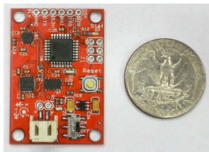
Fig. 5- An AHRS sensor board
