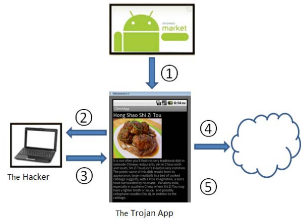
Fig. 1. Work Flow of a Premium SMS Android Trojan App in Our Mobile Malware Case Studies. (① the Trojan app is downloaded and installed on the victim's device; ② when the Trojan app is activated by the victim, it sends a notification with the victim's information to the hacker; ③ the hacker sends the commands to the Trojan app to ④ send SMS to premium numbers or send Ad SMS to others; and ⑤ the trojan app clears messaging history.)
