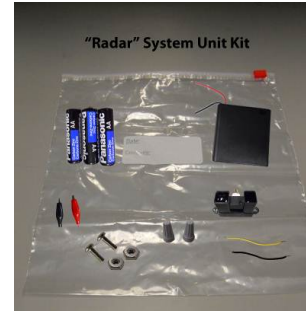
Fig. 2. A "radar" system unit kit is prepared for each group of students. The kit contains a battery holder, three AA batteries, a Sharp IR sensor, two alligator clips, two screws, two hex nuts, and two wire connectors.
