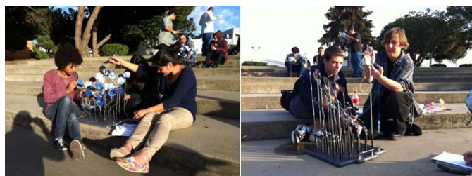
Fig. 2. The students are gathering data from their central tower concentrating laboratory set-ups.
